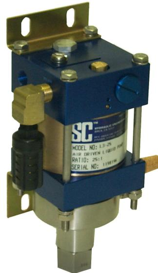
**SC** air driven compact liquid pumps operate on the principal of differential areas. An air piston drives a smaller diameter hydraulic plunger to provide a pressure ratio. The pressure ratio determines the maximum outlet pressure.
