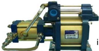
All SC air boosters are pre-lubricated at the factory and should not be used with inline air lubricators. Clean, dry air is very important as any grit, moisture, or foreign matter in the air supply can damage the high pressure components. A coalescing filter is recommended before the air supply and air drive inlet, which can be the same.
